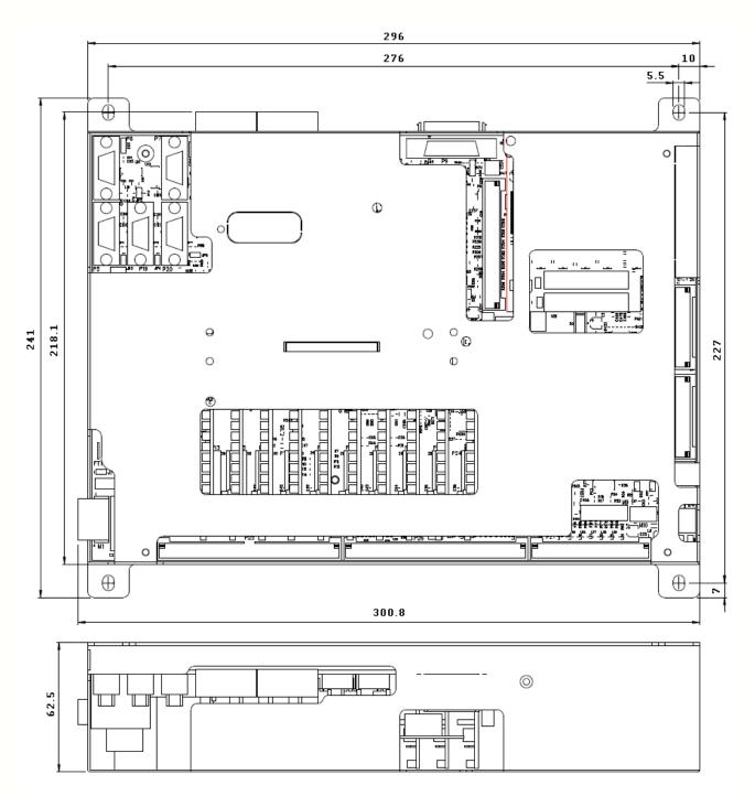
With FDC expansion board the overall height is 130 mm.
