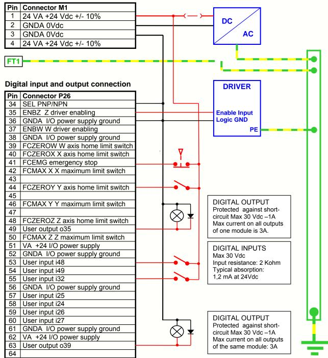
**NB:** CE regulations recommended to place the free-wheeling diode in proximity of each inductive load to prevent the spread of electromagnetic interference along the wiring cables.
