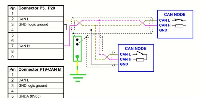
The same power supply voltage supplied to the controller is available between pins 5 and 9 of connector P19. This voltage can be used to supply external devices which do not absorb more than 100 mA.
