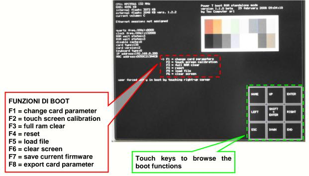
WARNING: the Boot menu only manages the USB memories and not any other peripherals, such as the keypad and the mouse, which may be connected to the same USB port by means of a hub.
